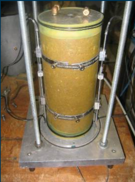
Bench-Scale Resilient Modulus Test
